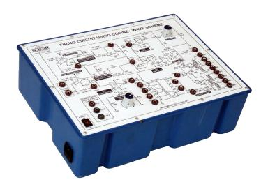
**OMEGA TYPE PET-425** Power Electronic Training Board has been designed specifically for the study of the firing circuit for single-phase converter using cosine-wave comparator scheme.
