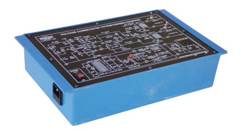
**OMEGA TYPE PET-430** Power Electronic Training Board has been designed specifically for the study of the step down voltage commutated thyristorised chopper.
