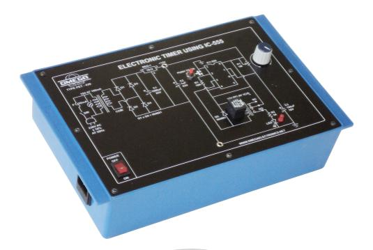
**OMEGA TYPE PET-439** Power Electronic Training Board has been designed specifically for the study of Electronic Timer using IC-555. The board is absolutely self contained and requires no other apparatus.
