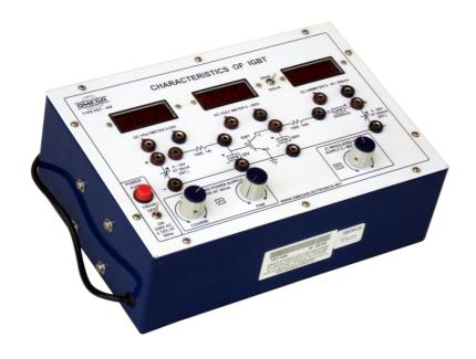
**OMEGA TYPE PET-449** has been designed specifically to study & Plost VI Characteristic of Power IGBT. The board is absolutely self contained.
