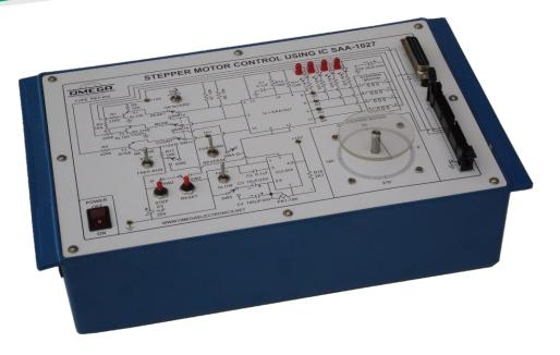
**OMEGA TYPE PET-450** Stepper Motor Control trainer are based on IC SAA-1027 & designed to study the various functions of a stepper motor. It can be interfaced with microprocessor trainer and personal computer.
