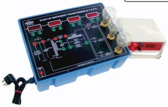
OMEGA TYPE PET-454 Power Electronic Training Board has been designed specifically to study the working and application of instrument transformer. Measurement of power using Current and Potential Transformers. The setup consists of current Transformer, Potential Transformer, Ammeter, Voltmeter, Watt meter, Variac and Actual Load.
