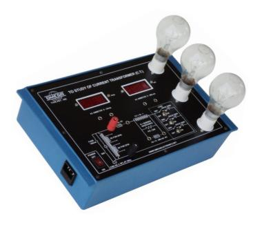
**OMEGA TYPE PET-452** Power Electronic Training Board has been designed specifically to study Current Transformer (C.T.).
