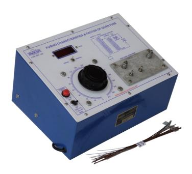
**OMEGA TYPE PET–456** Power Electronic Training Board has been designed specifically to determine the fusing characteristics and fusing factor of a given fuse.
