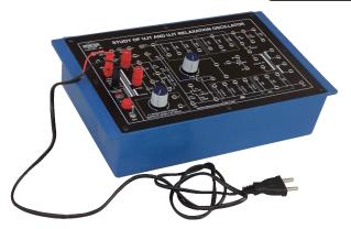
**OMEGA TYPE PET-401** Power Electronic Training Board has been designed specifically for the study of Electrical Characteristics of Uni-Junction Transistor. The UJTs are widely used for Relaxation Oscillator, waveform & pulse generators and firing circuits of SCR's and TRIAC's. This Training Board can also make use for designing firing circuits and control circuits for thyristors.
