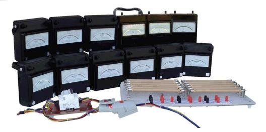
**OMEGA TYPE ES–334** Experimental setup has been designed specifically to verify the voltage and current relations in star and delta connected systems.
