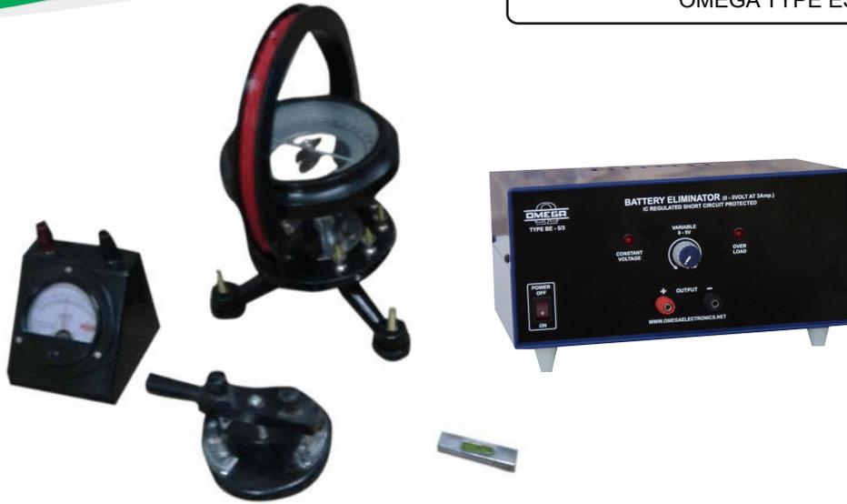
**OMEGA TYPE ES-226** Experimental Set Up has been designed specifically to determine the value of Horizontal Component of the Earth's field by using Tangent Galvanometer and an Ammeter.
