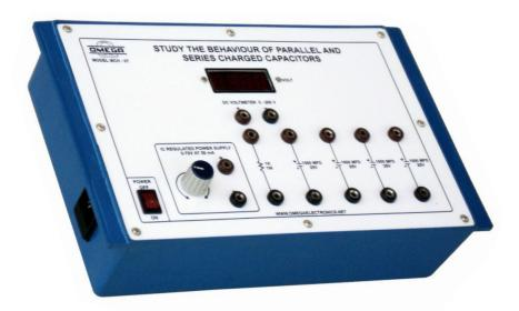
**OMEGA TYPE MCH-07** Experimental Training Board has been designed specifically to study the behavior of Parallel & Series Charged Capacitors.
