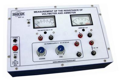
**OMEGA TYPE MCH-02** Training Board has been designed specifically for the Measurement of Resistance of Voltmeter and Ammeter. The board is absolutely self contained and requires no other apparatus
