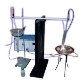
**OMEGA TYPE MCH-14** Experimental Set Up has been designed specifically for the Measurement of e.m.f. with Thermocouple Using Digital D.C. Micro voltmeter and Sand Bath. The aims are to plot thermos emf versus temperature graph and to find the melting point of Paraffin Wax using digital D.C. micro voltmeter and sand bath.
