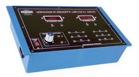
OMEGA TYPEL MCH-12 Experimental Training Board has been designed specifically to verification the Kirchoff's law for D.C. circuit.
