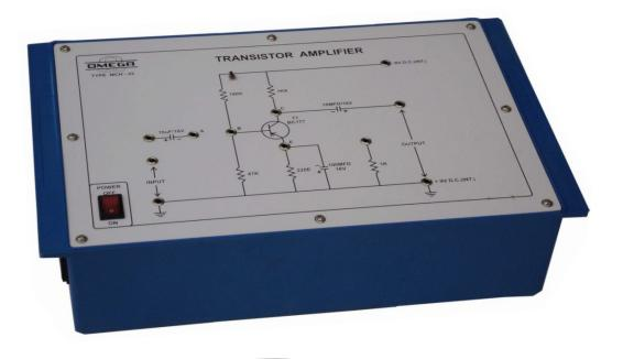
**OMEGA TYPE MCH-22** Experimental Training Board has been designed specifically for the study of voltage gain, frequency response, input impedance, output impedance, current gain, Power gain of a Common Emitter (CE) Transistor Audio Amplifier.
