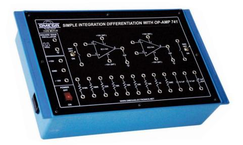
**OMEGA TYPE MCH-25** Experimental Training Board has been designed specifically for the study of OP-AMP IC's applications. This training board covers Integrator and Differentiator application of operational amplifiers (IC-741) and makes the student familiar with it.
