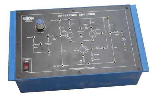
OMEGA TYPE MCH-21 Experimental Training Board has been designed specifically for the study of Differential Amplifier in solid state version. A Differential Amplifier is also called a Differential Amplifier and it is essential part of operational amplifier. As operational amplifiers are now a days being used quite extensively in instrumentation control and entertainment electronics, this Training Board has great educational value.
